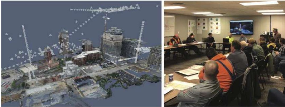
Figure 25.21 3D models of construction sites are produced from images by structure-from-motion and multiview stereo algorithms. They help construction companies to coordinate work on large buildings by comparing a 3D model of the actual construction to date with the building plans. Left: A visualization of a geometric model captured by drones. The reconstructed 3D points are rendered in color, so the result looks like progress to date (note the partially completed building with crane). The small pyramids show the pose of a drone when it captured an image, to allow visualization of the flight path. Right: These systems are actually used by construction teams; this team views the model of the as-built site, and compares it with building plans as part of the coordination meeting. Figure courtesy of Derek Hoiem, Mani Golparvar-Fard and Reconstruct, produced by a commercial system described in a blog post at medium.com/reconstruct-inc .
