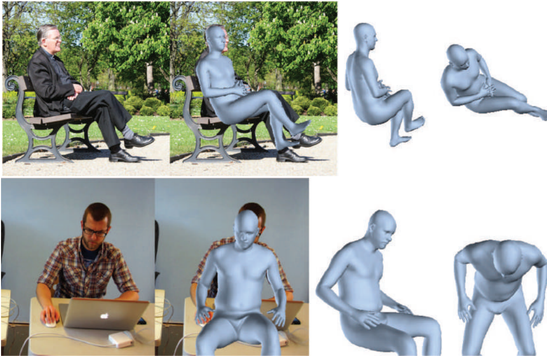
Figure 25.16 Reconstructing humans from a single image is now practical. Each row shows a reconstruction of 3D body shape obtained using a single image. These reconstructions are possible because methods can estimate the location of joints, the joint angles in 3D, the shape of the body, and the pose of the body with respect to an image. Each row shows the following: far left a picture; center left the picture with the reconstructed body superimposed; center right another view of the reconstructed body; and far right yet another view of the reconstructed body. The different views of the body make it much harder to conceal errors in reconstruction. Figure courtesy of Angjoo Kanazawa, produced by a system described in Kanazawa et al. (2018a).
