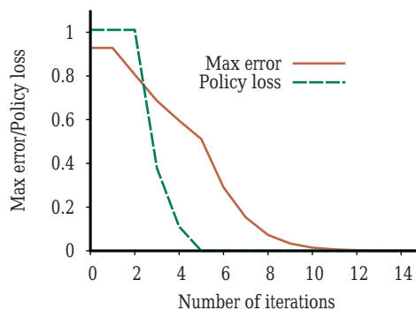
Figure 17.8 The maximum error \|U_i - U\| of the utility estimates and the policy loss \|U^{\pi_i} - U\| , as a function of the number of iterations of value iteration on the 4 \times 3 world.
